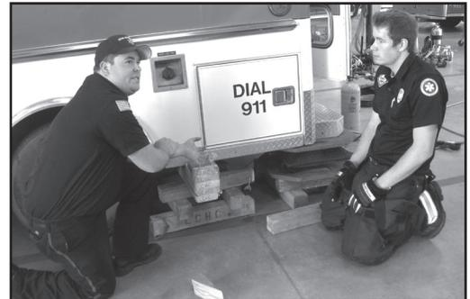
**Stabilize the Load:** Wood blocks are placed under and around the lifting bag to support the raised vehicle, as shown by Brock and Firefighter/EMT Jeff Carey.
