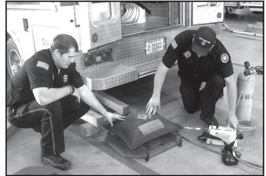
**Lift the Load:** Firefighter/EMT Tyler Hundt lays out pneumatic lifting bags, which are made of aramid-reinforced rubber (left). The largest bag lifts 26.5 tons to a height of 12 inches. Paramedic Richard Brock (right) operates a control that inflates a lifting bag with air.
